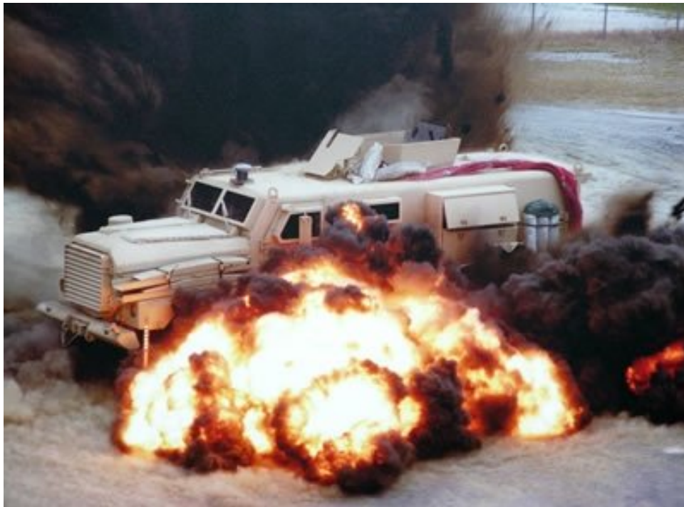
Picture 3 An MRAP COUGAR He tested in January 2007, with landmines detonating around it. 4
