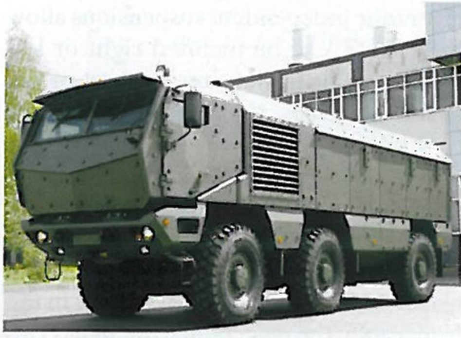
Picture 7 KAMAZ answered this requirement with the Typhoon mine protected truck That can host up to 18 soldiers 8
