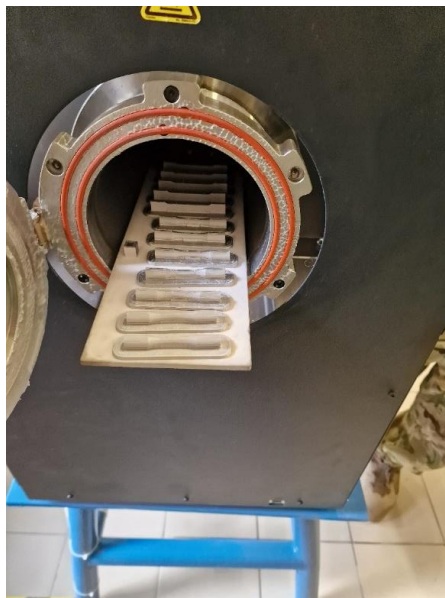
Figure 4. Manufacturing of standardised material test specimens
