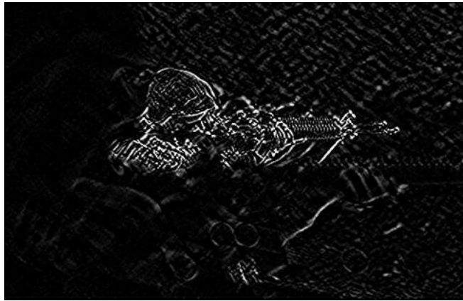
Picture 9 Canny edge detection of military objects: segmented data through online free software: Source: Wikimedia Commons: free open license
