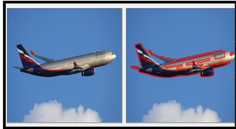
Picture 3 Canny edge detection of military objects: On the left: original data, on the right: segmented data through our software used edge detection
